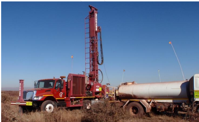
Figure 2: Booyesen Bore Schramm T 450 percussion drill
